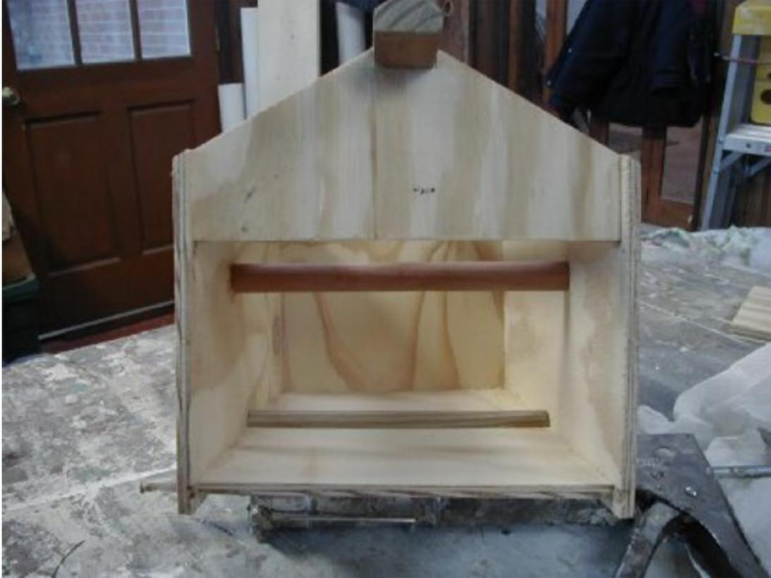
**The mounting of the chalet will allow for a slight forward tilt to the horizontal to let any water that comes in through the entrance hole to flow to the front and escape. To prevent the nest trays, if used, from sliding forward due to the slope and vibration or rack movement, I glued a small 3/8" by 3/8" strip at 6 1/4" from the rear. A nest tray can easily be lifted over this strip for inspection.**
