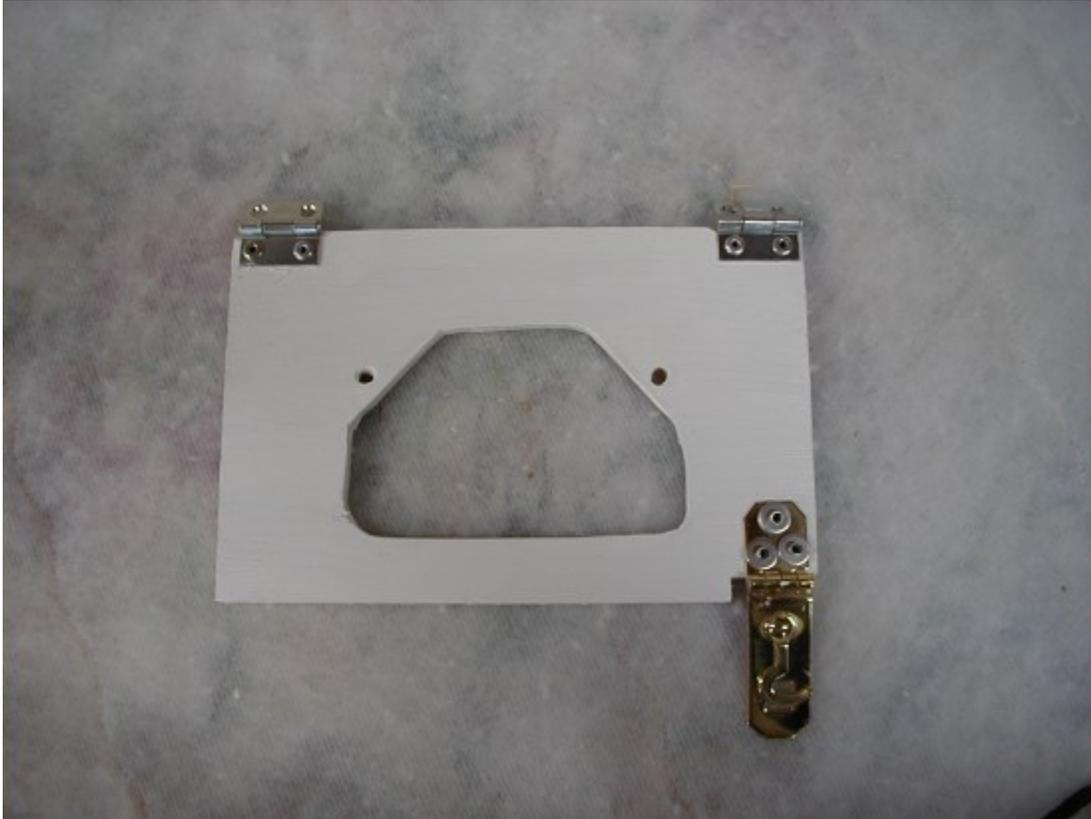
**I like to prime and paint before attaching fixtures to give added weather protection in that area. The hinges and clasp are placed at the ends of the door to give maximum room for any prefabricated entrance holes. The holes could easily be cut directly in to the door, but this would reduce the flexibility of changing entrance types.**
