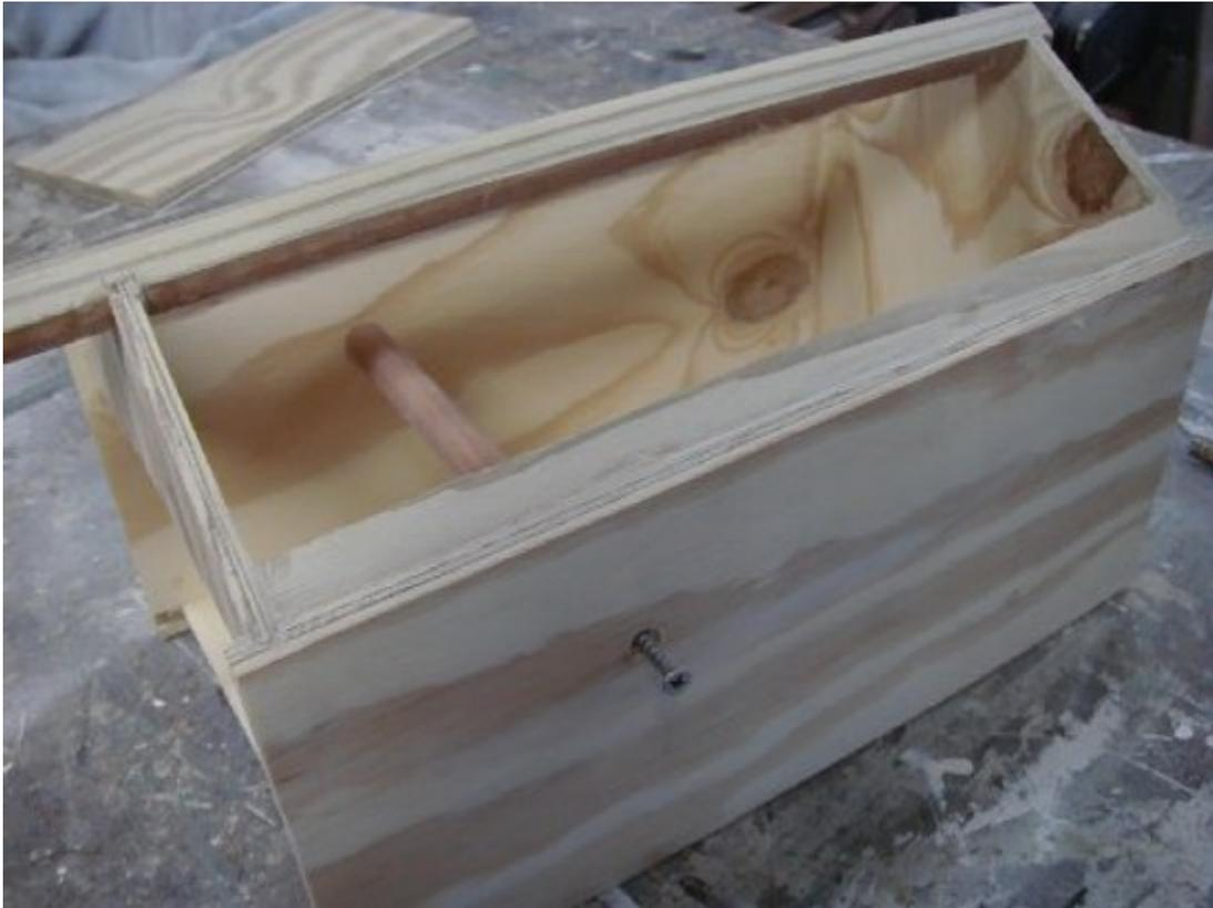
**Recent nest cam video has shown birds clinging to the sides of gourds and inspection ports while sleeping. Since the roof is high for ventilation, there is enough room to attach a perch. This is located 4" back from the opening and 4" from the floor. A 1/8" hole is drilled in the walls and countersunk. The ends of a piece of 5/8" dowel are also predrilled. The perch is attached to the sides by a deck screw.**
