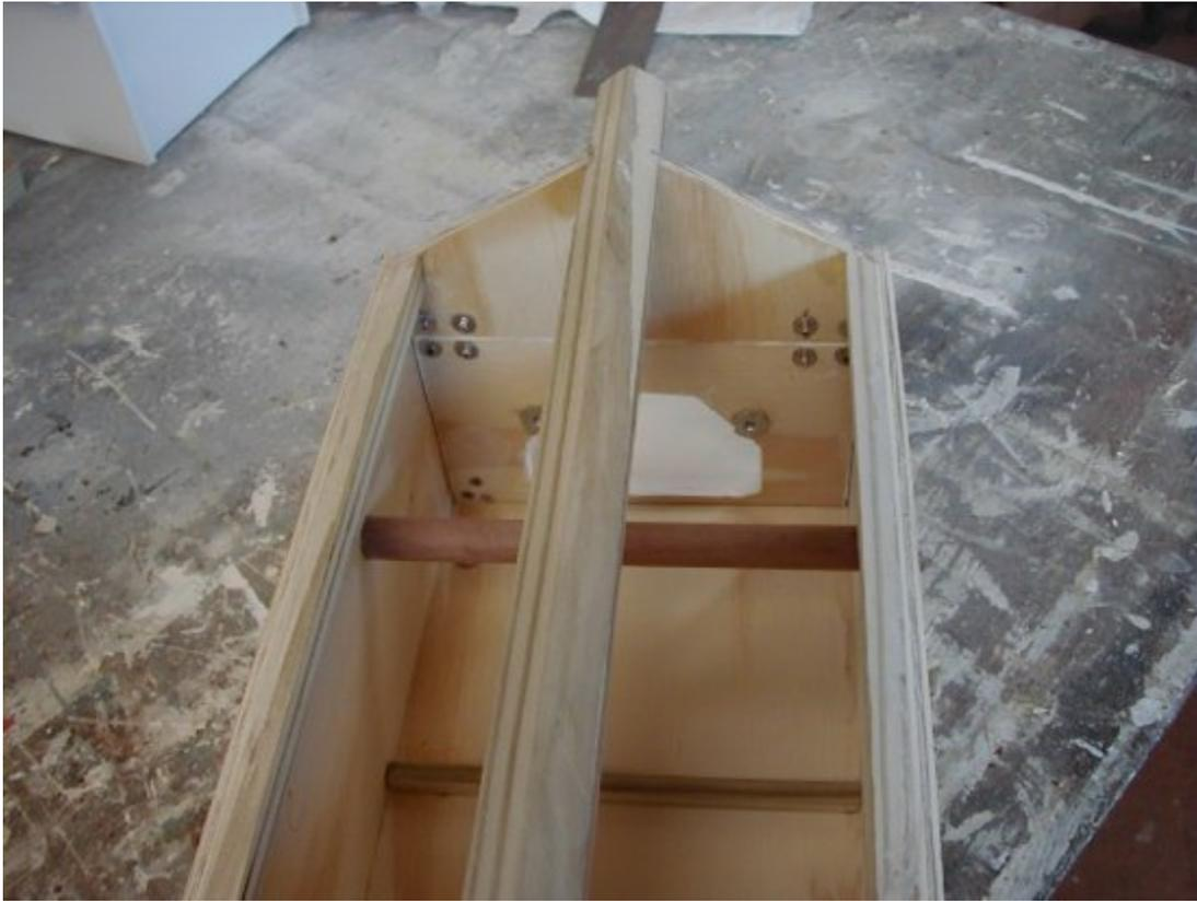
**The view of the back of the front panel shows the “T” nuts, perch and nest tray restrainer in place in place.**
