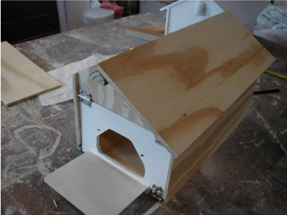
**Each roof panel should be marked with the location of the support beams to give a better guide when tacking the roof in place.**
