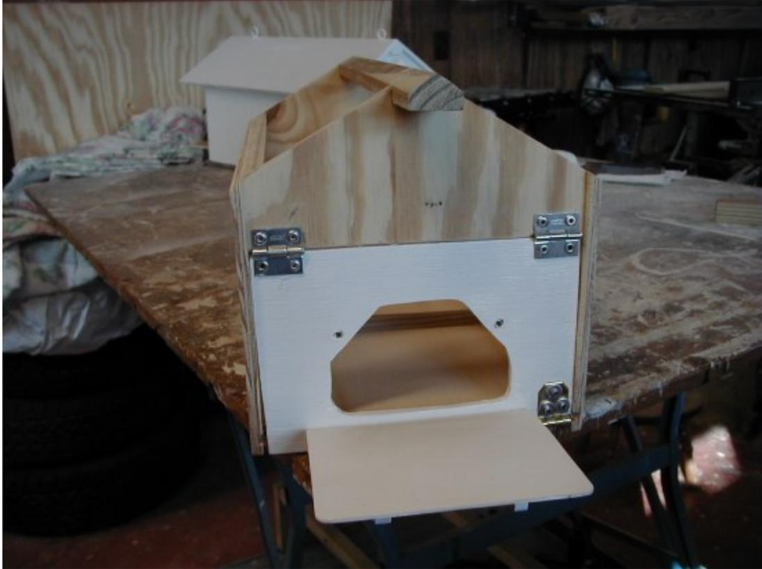
**The hinges and clasp are attached with pop rivets and backing washers since the door is only 1/4" thick, it would not hold screws well. When setting the rivets, if the force needed to pop them appears to be too great and the rivet looks to be set well enough, release the pressure and drive out the pin in order to prevent splitting the edge of the door. A small amount of material may have to be removed from the door and shell edge under the hinge barrels to let the hinge lie flat.**
