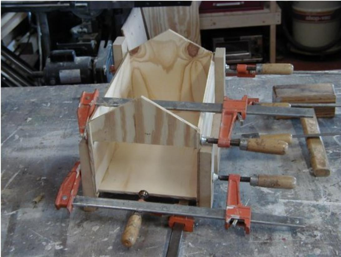
**At this time, all of these panels, except for the roof, are glued and clamped using PL premium polyurethane construction adhesive (PPCA) and allow to set for 24 hours.**
