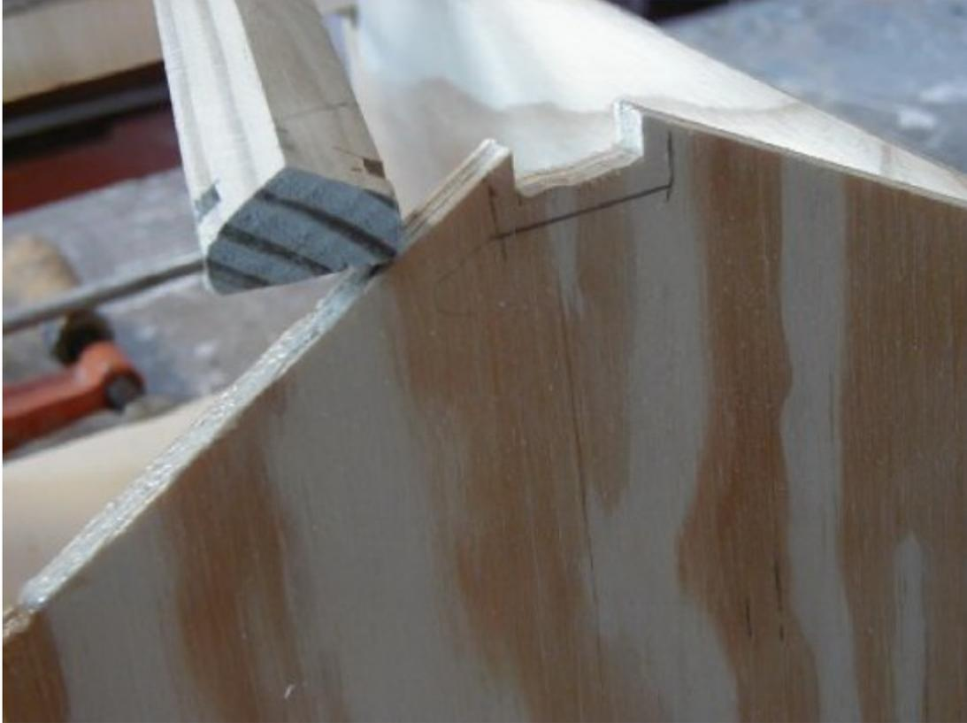
**For the ridge beam and eaves support, prepare two pieces of pine (I used pressure treated scrap) to be 1" wide and 5/8" thick and 14 1/2" long. Setting the saw at 30 degrees, trim off the shoulders to give the profile shown.**
